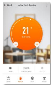
If you failed to pair, click "Retry" in SmartLife App. Long press the "M" button (5) on the control box to reset the pairing mode of the heater, following the directions in the SmartLife App.
