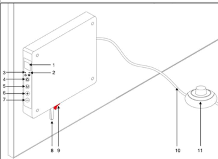
1. LED display showing setpoint temperature
