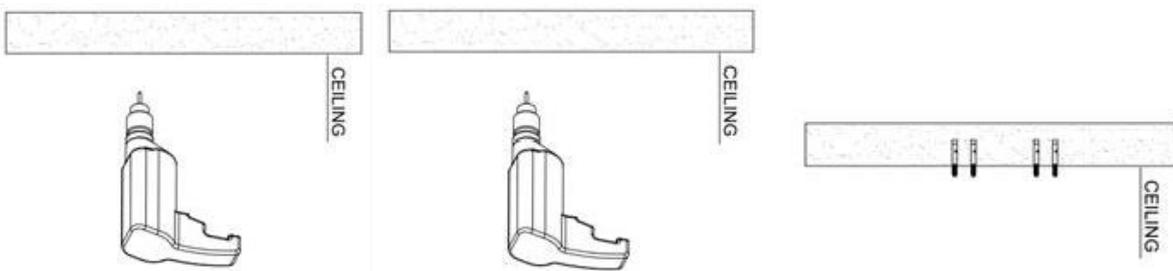
A wall mounting bracket is provided with the heater, which has been specifically designed to allow this product to be attached to a wall or ceiling. Before drilling the holes for the wall or ceiling mount, check that the surface is solid and that there are no hidden water pipes or electric wires. The heater must be installed no less than 40cm from any side walls and no less than 180cm from the floor.
