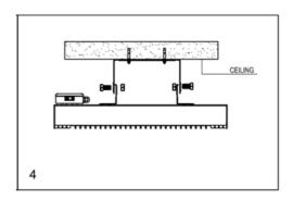
A wall mounting bracket is provided with the heater, which has been specifically designed to allow this product to be attached to a wall or ceiling. Before drilling the holes for the wall or ceiling mount, check that the surface is solid and that there are no hidden water pipes or electric wires. The heater must be installed no less than 40cm from any side walls and no less than 180cm from the floor.
