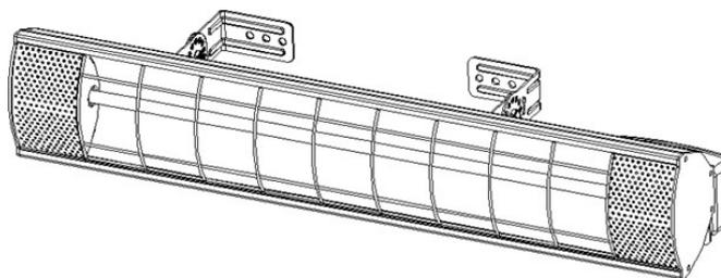
1. Fasten the brackets (1) together using the screws (6), washers (5) and wing nuts (4). (See Fig 1-2).
